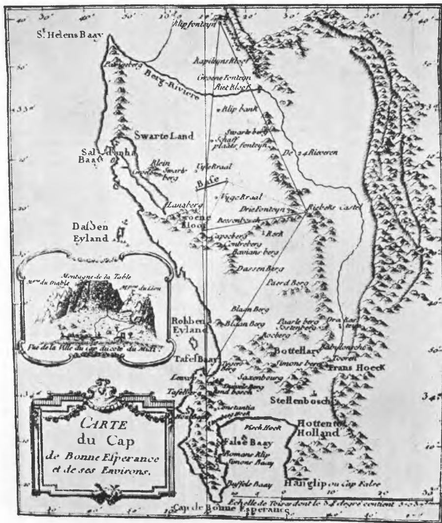
VII. Lacaille's map of his triangulation for measuring an arc of meridian. From his Journal historique , 1763.
