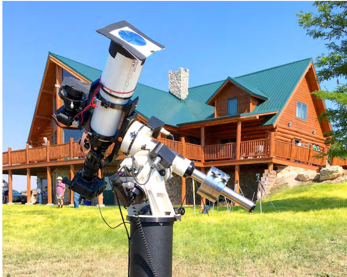
The author's eclipse imaging configuration – Custom APM 115/805 with 3" Feather Touch focuser and Takahashi flattener-reducer. This normally produces an effective f/5 , but here the polariser slightly constricts the aperture so the system aperture was f/6 . The mount is an Astro-Physics 900GTO. The primary camera is a Canon 5D Mk II. The piggy-back camera mounted on top of the refractor is an unfiltered Fujifilm X-Pro2 with OM 500/8 mirror-lens and Metabones focal reducer. The backup camera was only exposed during totality.
