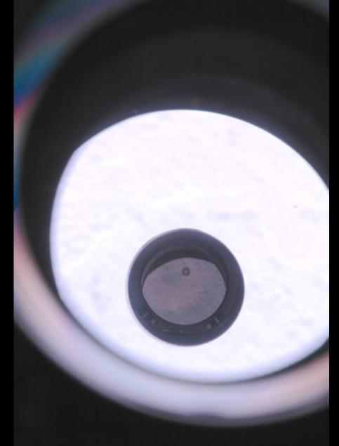
View down focuser tube looking onto secondary with image of primary shown as large white disc. Image taken to indicate relative size of secondary obstruction. Reflection of secondary seen inside darkannulus in centre. Primary is fully visible inside secondary at full back focus 4.5" above OTA tube.
