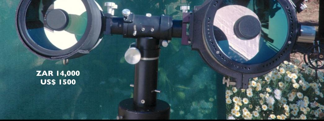
Santels are very rare Maks that were produced by Alaxei Santel in 152, 180, & 229 mm apertures (7, 8, 9") for about three years in the early 2000s. His craftsmanship was meticulous. Despite the solid all-metal build, this scope weighs only 8 kg. The built-in focuser is shift-free and ultra-precise.
