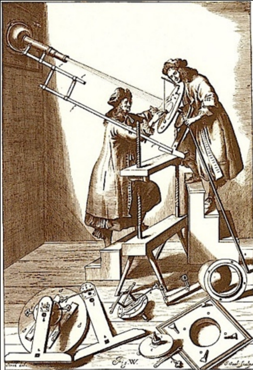
Equipment used by Hevelius with a telescope to project an astronomical image onto a sheet of paper. This arrangement was used in his historic observation of the transit of Mercury on May 3, 1661.
