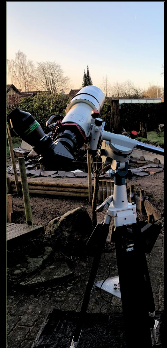
ZEISS (CZJ) 4" Refractor Model APQ D100/F640 ZEISS Ib Motorized Mount & Tripod
