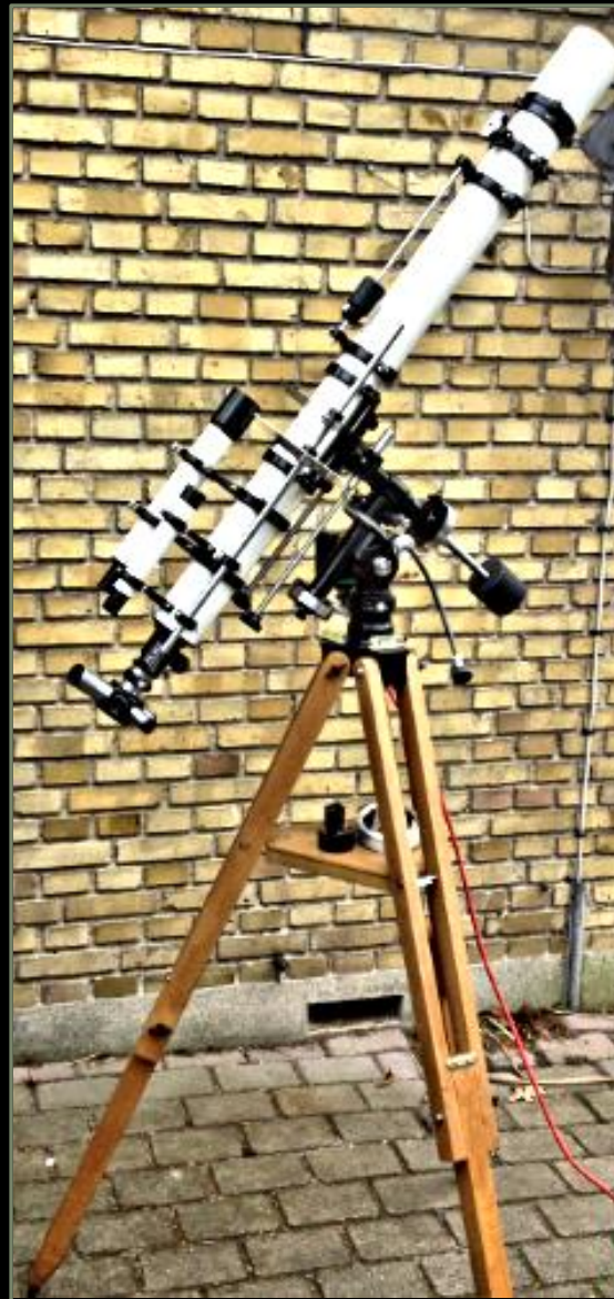
UNITRON (POLAREX) 3" Refractor Model 142, D75/F1200 UNITRON Motorized Mount & Tripod
