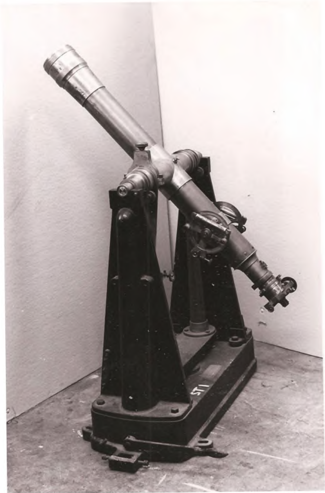
The Troughton & Simms Transit telescope on its cast-iron stand. (Courtesy - Local History Museum, Durban)
