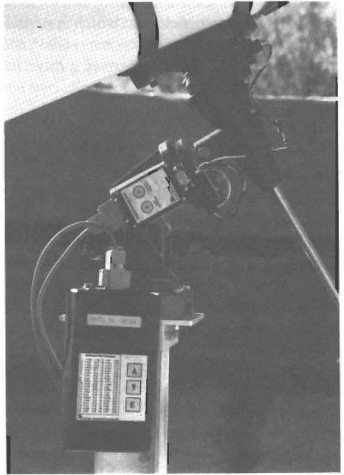
Figure 3. The complete encoding system installed on a German equatorial mount.
