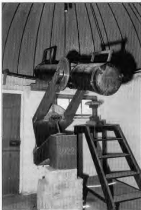
Forbes' 210mm Newtonian. Note the astronomers steps and adjustable seat in the background.
