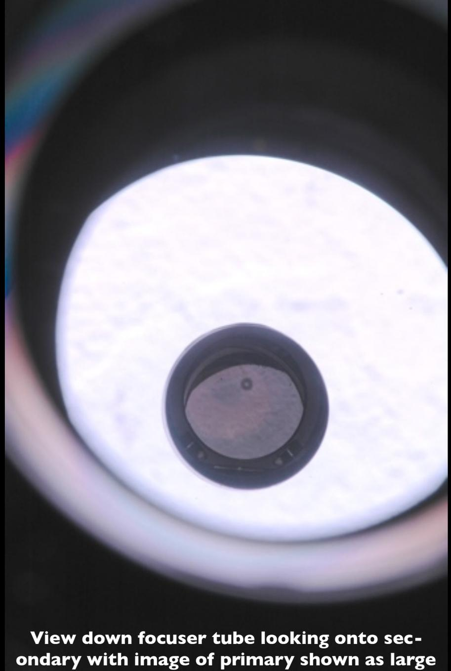
**View down focuser tube looking onto secondary with image of primary shown as large white disc. Image taken to indicate relative size of secondary obstruction. Reflection of secondary seen inside darkannulus in centre. Primary is fully visible inside secondary at full back focus 4.5" above OTA tube.**
